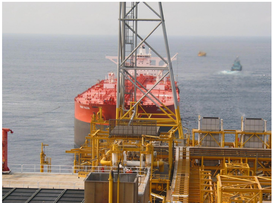
Example of tandem offloading operations
